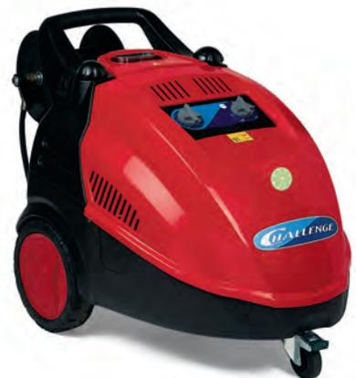
**Pressure Washer, Challenge 1500 PSI,** is a self contained hot water high pressure washer. It has long life components in the pump and motor for reliability. The controls are easy to reach. The motor is 2 pole, continuous duty, air cooled with thermal cutout. It offers an auto-feed anti-scale tank with a 3.2 gallon detergent tank. IPECHALL Pressure Washer, Challenge 1500, 2.1 GPM
